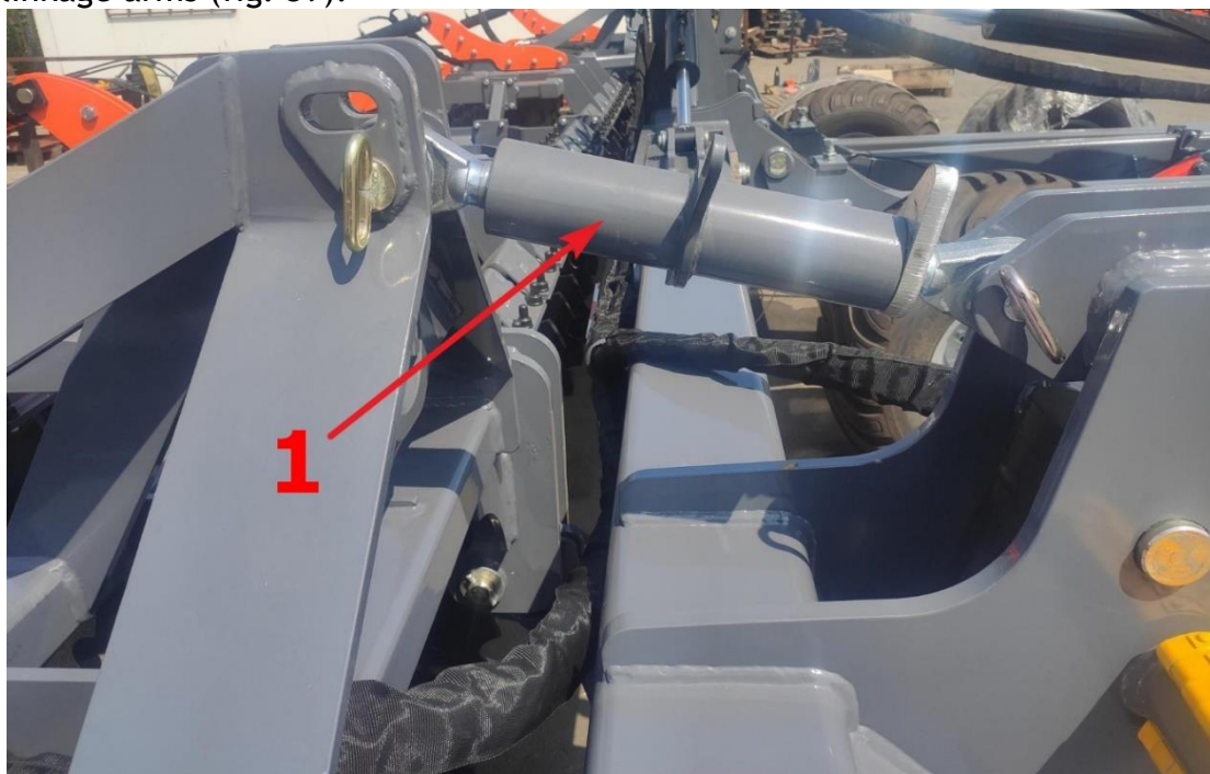
Figure 39 Placing the turnbuckle on the drawbar assembly; 1- turnbuckle.
