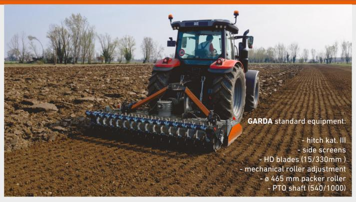
Mandam **GARDA** is a heavy-duty power harrow built to prepare the ultimate seedbed with exceptional efficiency. Its robust 12mm reinforced steel chassis and solid tungsten-steel tines deliver unwavering performance in both compacted and challenging soil conditions. Double blade rotors with 3 reinforced bearings and elongated splined shaft overlap provide an outstanding stiffnes and durabulity. Rotor stone protection is a standard equipment.
