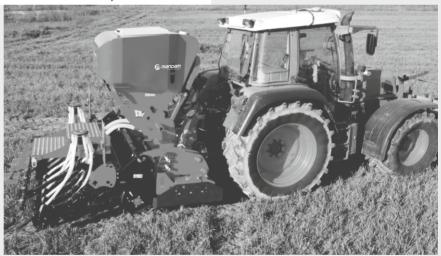
Available as a **GARDA COMBO** - a combination of power harrow and a pneumatic seeder unit.
