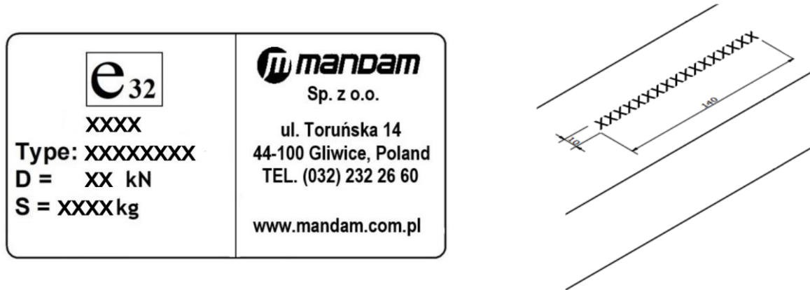
Figure 5 Example of the nameplate of an approved machine and the VIN number.
