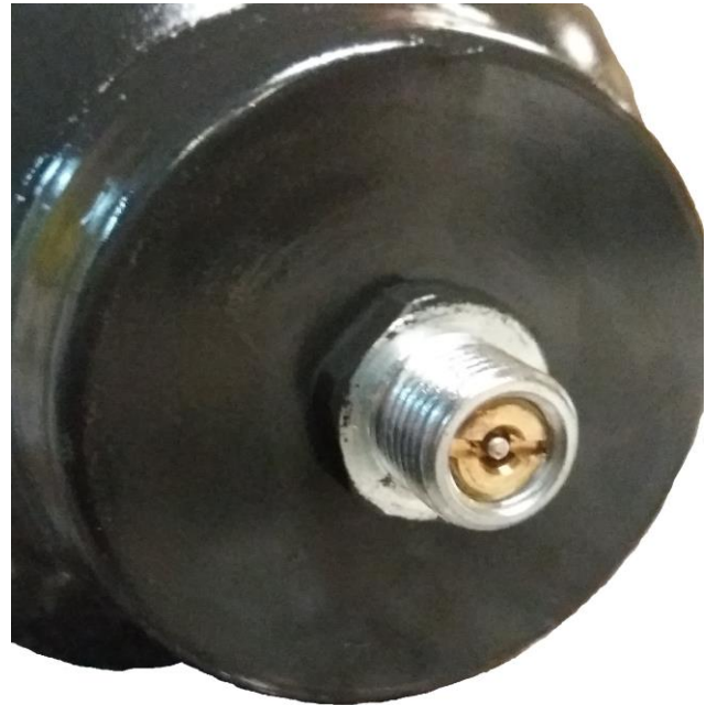
View of the pressure control valve
