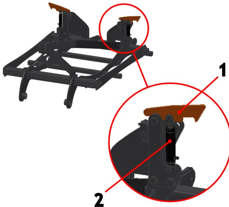
Figure 7 Projection central frame of cultivator with automatic wing locking mechanism (1 - hook of mechanism, 2 - actuator)
