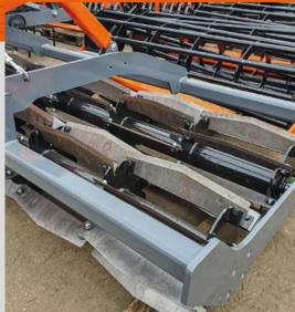
WNT TANDEM KNIFE ROLLER is a machine designed for intensive shredding of plant material (straw, crop residues, stubble, catch crops) along with crushing and partial covering. This accelerates the decomposition of residues, which facilitates further work on crops.
