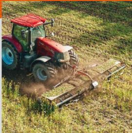
WNT HD TANDEM knife roller is a reinforced version of the standard WNT machine designed for work in the most difficult conditions, equipped with a double ø560 mm roller and HARDOX guillotine knives. The top cover is standard. The purpose of the roller is intensive shredding of plant mass along with crushing and partial covering. This accelerates the decomposition of residues, which is conducive to further work on post-harvest crops. The working depth of the machine is 2-3 cm (knife depth).
