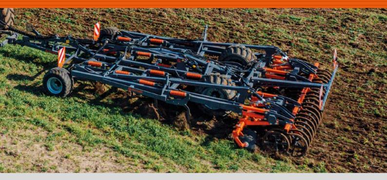
The RHINO CHISEL CULTIVATOR is designed for stubble (up to 12 cm) and no-tillage cultivation (up to 35 cm depth). Available at working widths of 4.50 m and 6.00 m. The use of right- and left-side moldboards increases the intensity of stubble mixing, which reduces the intensity of phenolic compounds that negatively affect the development of cereals in the following year.
