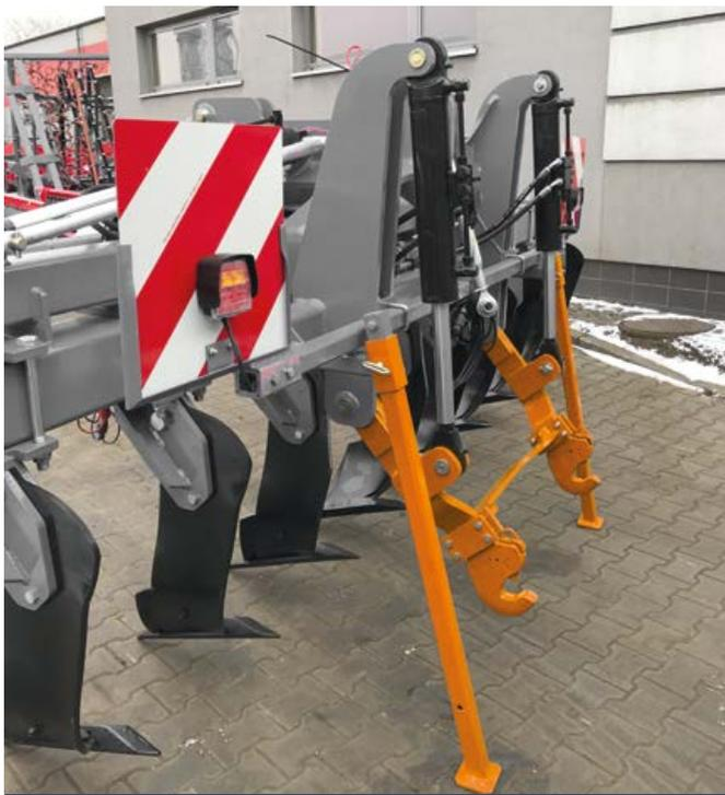
**ATTELAGE HYDRAULIQUE AVEC CROCHETS (MGPH)**
