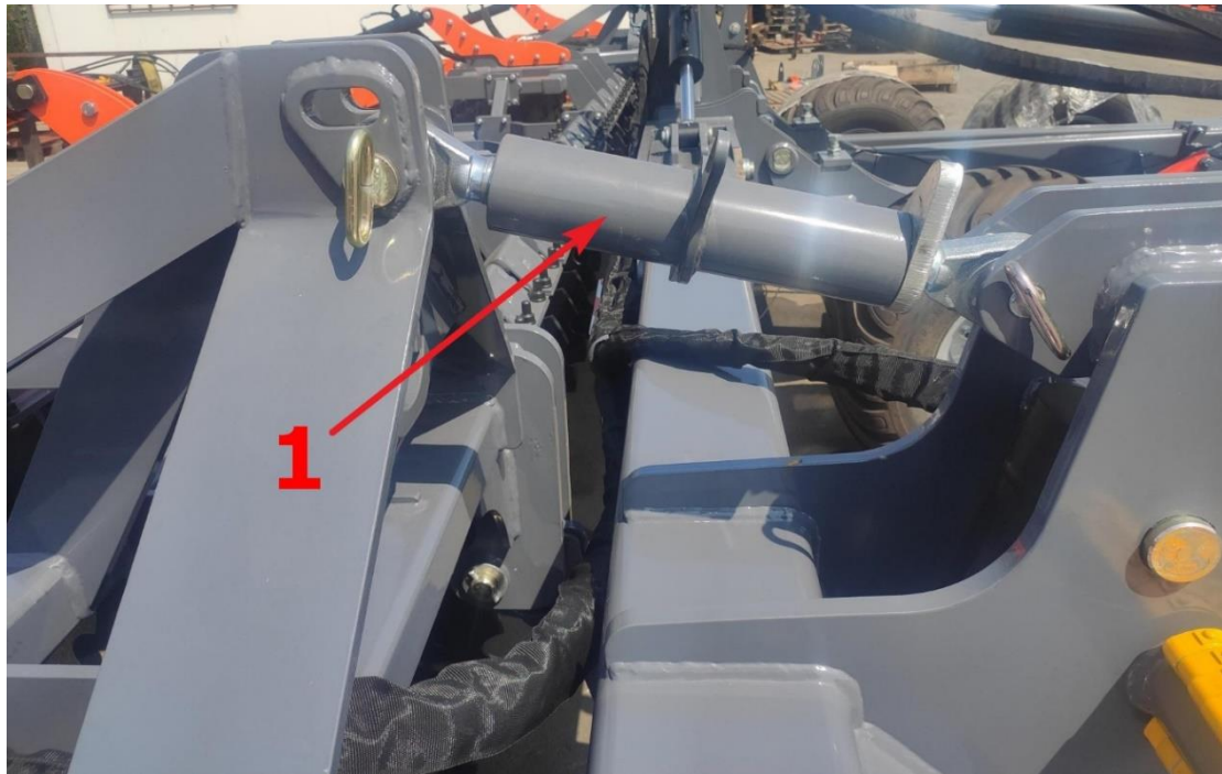
Fig. 25 Placement of turnbuckle on drawbar assembly; 1- turnbuckle.
