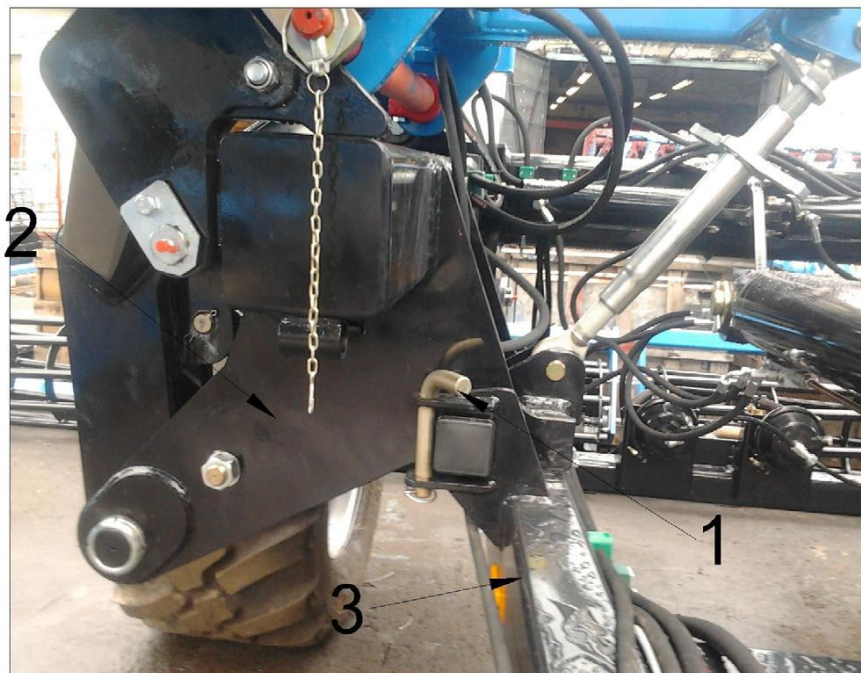
Fig. 5 Arm lock for the sections in TAL-K 8,0: 1 – locking device, 2 – section arm, 3 – carriage frame
