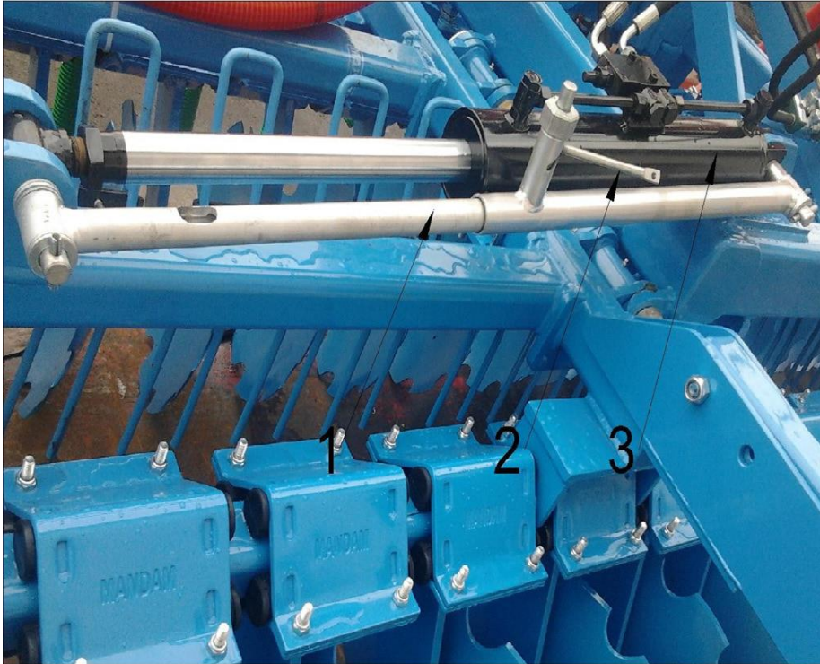
Fig. 3 Mechanical lock in TAL-C: 1 – mechanical protection, 2 – cord-pulled lock arm, 3- cylinder
