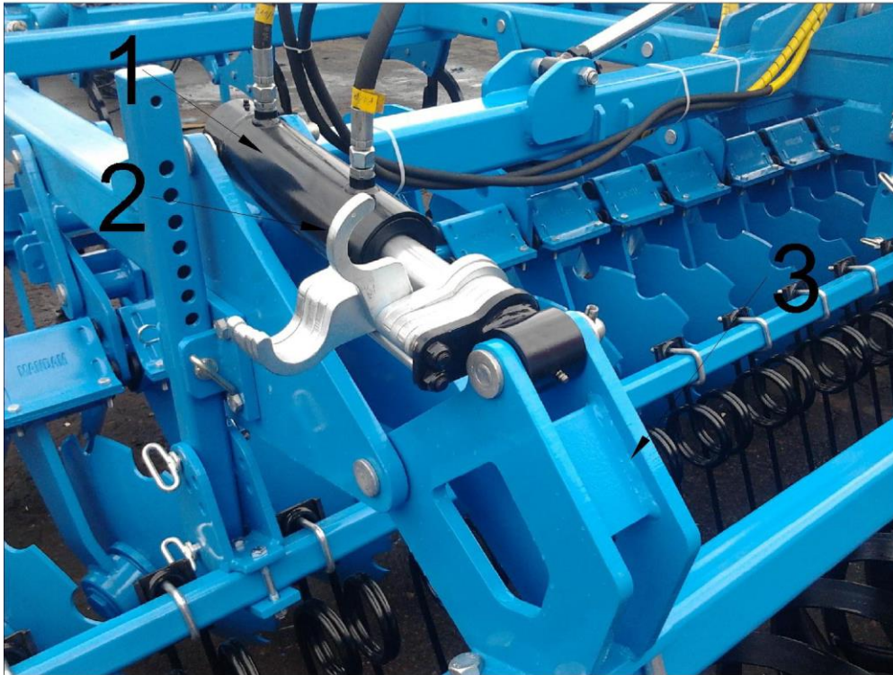
Fig. 8 Hydraulic adjustment of the shaft depth 1 – cylinder, 2 – latches for adjusting the working depth, 3 – shaft arm
